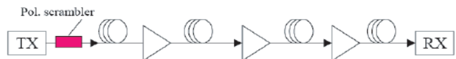
Figure 2. A 2540P Polarization Scrambler application for PDG mitigation. Without polarization scrambling, the finite amount of the DOP from the signal source results in different receiver signal intensity due to PDG.
